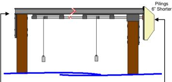
8" pilings need to be installed with sufficient seabed penetration to support the weight of the boat. Pilings must be square and level to each other. The two drive end pilings (the pilings where the hoists are mounted) should be 6" shorter than the 2 other pilings. ANY movement of the pilings after installation will adversely affect lift operation and safety.
