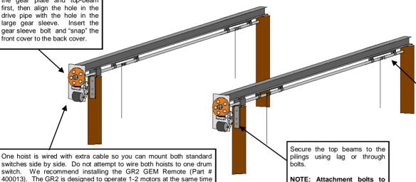
All 4 cable pieces must be equal in length. When attaching the cable to the pipe, insert the unfinished end of the cable into the hole of the drive pipe. Feed it through the pipe shaft and out the end of the pipe. Attach the 1/4" cable clamp to the cable and pull the cable back through. Make sure the clamp is tight inside the drive pipe.
