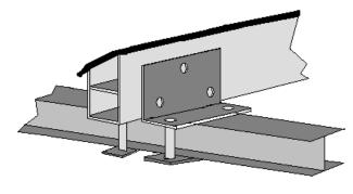
Aluminum bunks are mounted to the I-Beams using 8 pc of 6" x 4" un-even leg angle, each pc will have three holes punched in them. Set the bunk in the desired location flat on the beam and place one angle on each side. Drill through the bunk and through bolt using all three holes. Next attach the bunks to the cradle using the long SS bolts and the flat back up plate. End caps are supplied with the bunks and press in the ends.
