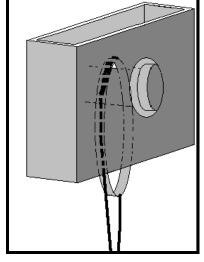
Insert the 5/8" x 3" Stainless Steel bolt through the inside channel in hole center with cable winder then through the 1" x 2" aluminum tubing. Using the 5/8" thimble, make a loop with the cable, slide the bolt through the thimble and out the other side of the tubing. Make sure you use the flat-washers to help distribute the forces. Secure with the stainless steel nut.
