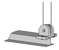
10K and larger lifts are compounded or double lined lifts. The I-Beam clamps will include a sheave for compounding, simply run the included cable around the sheave and straight back to
