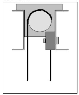
When compounding make sure that the start of the cable wraps on the outside of the lift and the compounding bracket is bolted to the inside beam. This will insure that the dead-end bracket will not interfere with the winding of the cable on the drive pipe.
