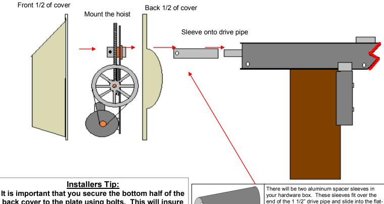
It is important that you secure the bottom half of the back cover to the plate using bolts. This will insure that the cover will snap into place. You will also need to notch the cover where you would like the control cable to come out, we suggest the bottom.
