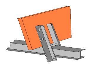
Wood bunks are mounted to the beams using 8 Pc of long angle (length of angle depends on Lift) each angle will be a set (right and left) Wood bunks need to be angled into the boat for strength. Boat Hoist USA does not supply the wood for the bunks but recommends using a hard, treated lumber at least 10" and 12' long.
